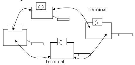
Each node is connected to two (2) others forming a ring.
