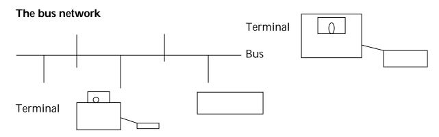
In the bus network, each device handles its own communication control. There is usually no host computer or file server. A file server is a large capacity hard disk storage device and it basically stores data and programs.
