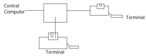
A number of small computers or peripheral devices are linked to a central unit. The central unit may be a host computer or a file server. A host computer is a large centralised computer, usually a mini computer or a main frame. This topology is common for linking several micro computers to a main frame.
